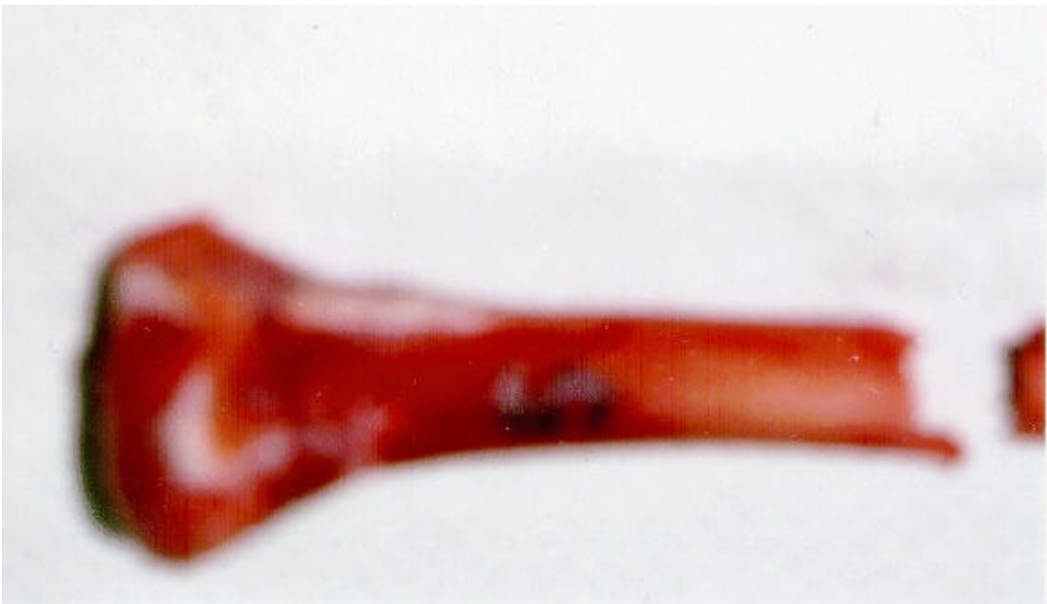
Figure 6. Enlarged picture of a chicken bone fractured using three point bending Instron. The bone fractured along the transverse cross-section (perpendicular to the longitudinal cross-section).
