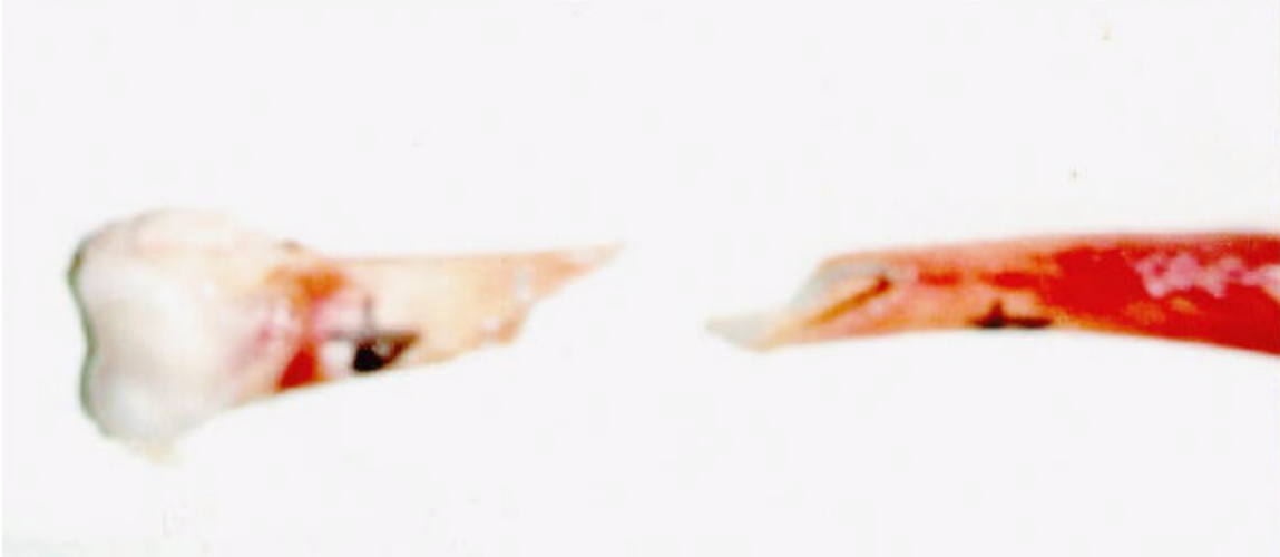
Figure 5. Enlarged picture of a chicken bone fractured using impact pendulum. The bone fractured at an angle from the transverse cross-section.
